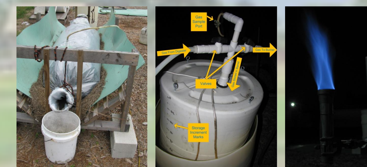
From left to right: working bag digester model, model gas collector, and biogas flame at night
