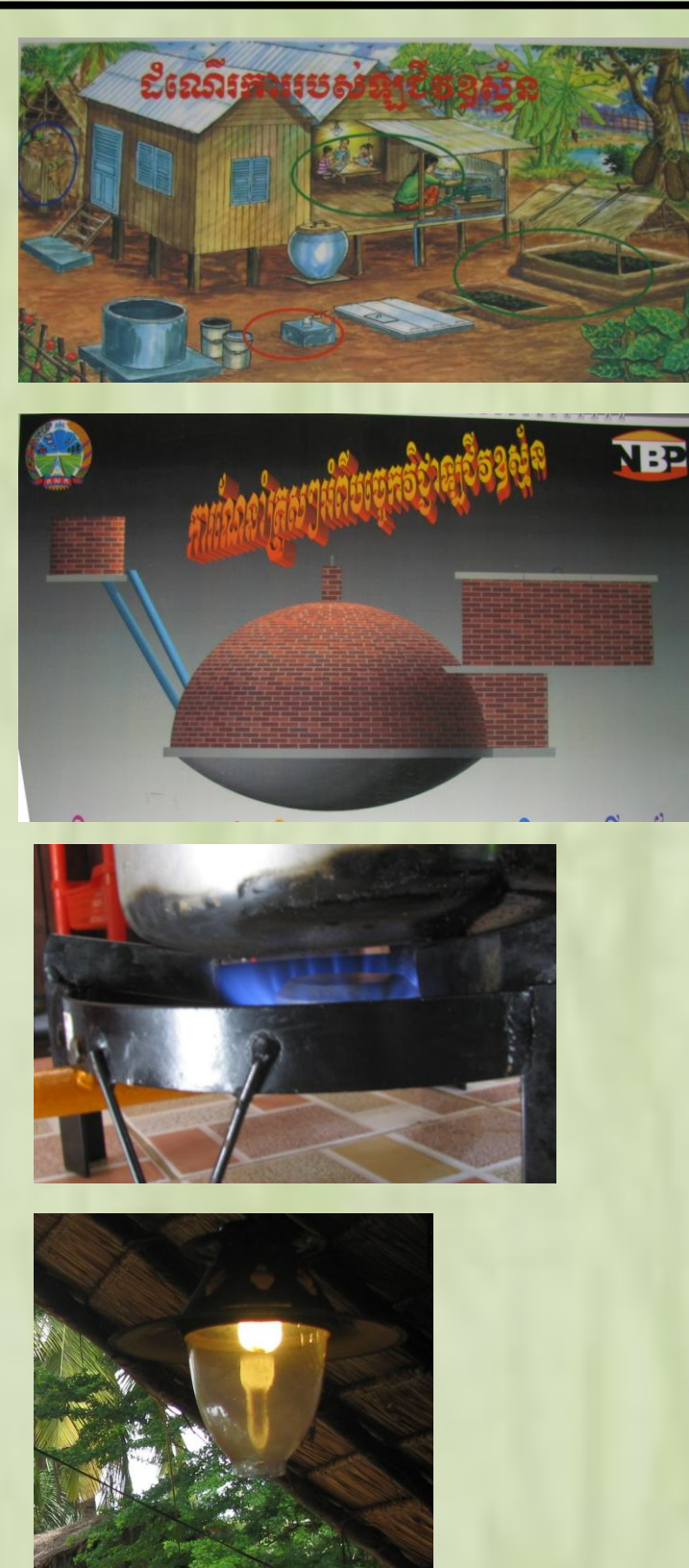
From top down: Artistic rendition of family home with digester, side view of NBP digester illustrating underground portion, stove running on biogas, lantern running on biogas.
